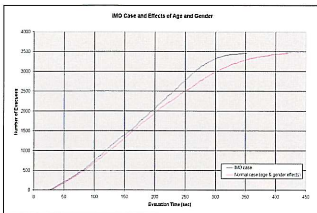
Fig 13. Case 1 – Basic IMO and normal cases. This shows a 20% increase in time due to gender and age. Both normal and IMO cases, however, suggest times for evacuation towards the lower end of the data provided in Ref 2.
