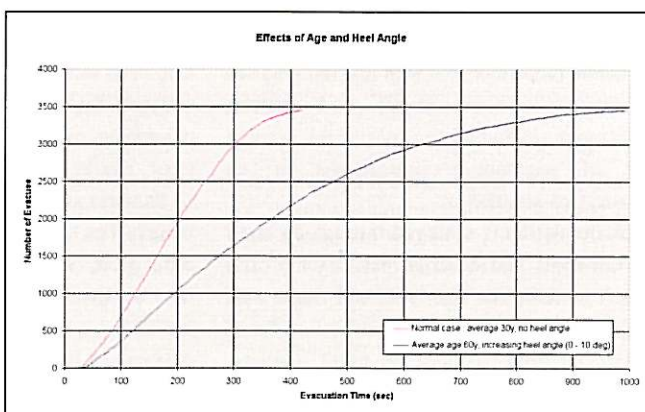
Fig 15. Case 5 – Effects of age and heel angle. The effect of this is to more than double the evacuation time. For comparison purposes, the opposite extreme is also simulated, referring to a mustering scenario where all the passengers are young (thus, faster walking speeds and shorter reaction times).
